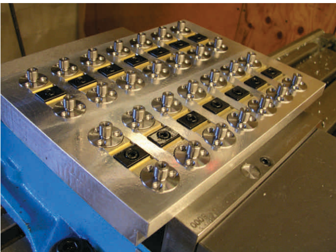
Fixtured with Mitee-Bitee Machinable Uniforce® Clamps
