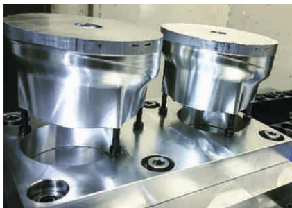
Loc-Down® 1/2-13 - Part No. 11500 M12-1.75 - Part No. 11612
