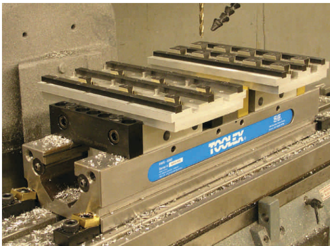
Fixtured with Mitee-Bitee Uniforce® Clamps and locating rails
